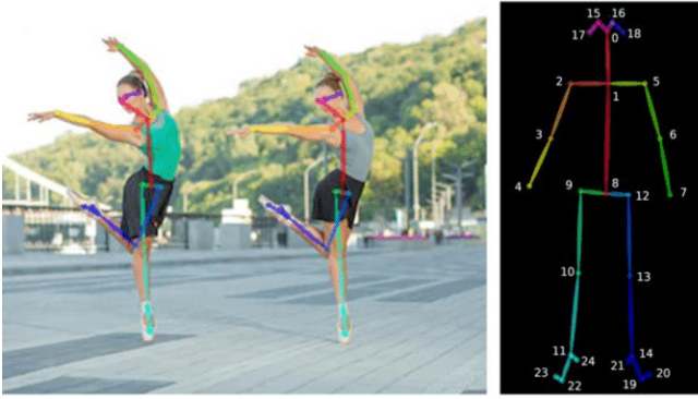
Figure 2: Multi-person Pose Estimation with OpenPose [30].
