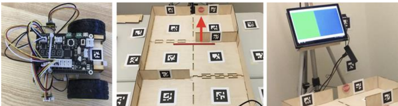
Figure 1. Materials used in the study: the robot that participants had to program (left), one example maze (middle) and the Kinect-based speech visualization (right).
